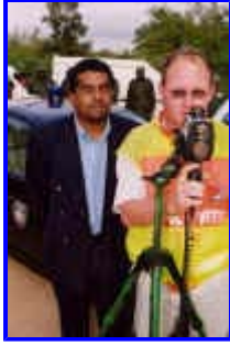
While KNP Protection Service head Mr Prego Reddy looks on, traffic officer Mr Dawie Botha takes aim with one of the KNP's Ladar speed measuring devices.
